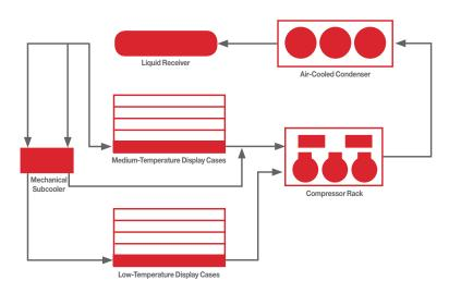
**Above:** In a full-scale supermarket refrigeration experimental evaluation under controlled laboratory conditions at Oak Ridge National Laboratories, Solstice N40 increased system COP by 11.6% and capacity by 7.5% over the ambient temperature range.
